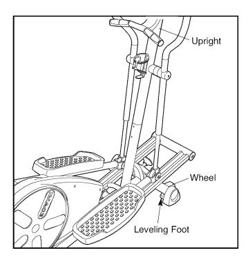
If the elliptical exerciser rocks slightly on your floor, turn one or both of the leveling feet under the front stabilizer until the rocking motion is eliminated.
